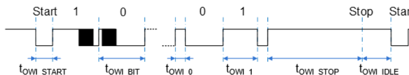
Figure 21. OWI Timing Diagram
